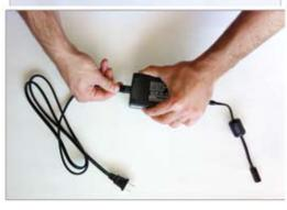
Plug input power cord into short transformer cord.
