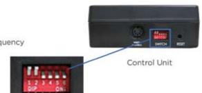
If installing two beds together, each with it's own remote control, make sure that bed A remote and control box are set to one frequency, and bed B remote and control box are set to another frequency.
